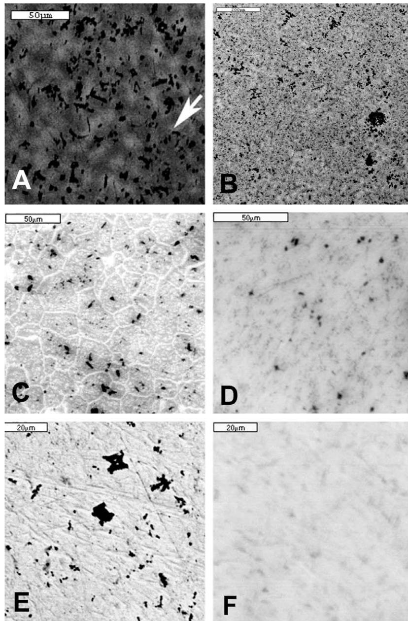
**Fig. 1.** Sample microstructures of the AFC-1 and AFC-2 alloys. The letter in each photomicrograph corresponds to the alloy composition listed in Table 1. All images were taken in backscattered electron mode in a scanning electron microscope. The black, globular inclusions in each photomicrograph are the oxygen-stabilized  $\alpha$ -Zr phase.
