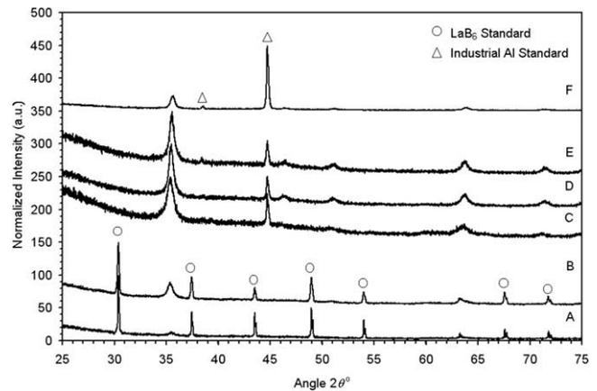
Fig. 4. X-ray diffraction patterns for the AFC-1 and AFC-2 metallic fuel alloys measured with either LaB<sub>6</sub> (SRM 660a) or industrial Al internal standard. Alloy-A is at the bottom, and alloys progress accordingly to F at the top.
